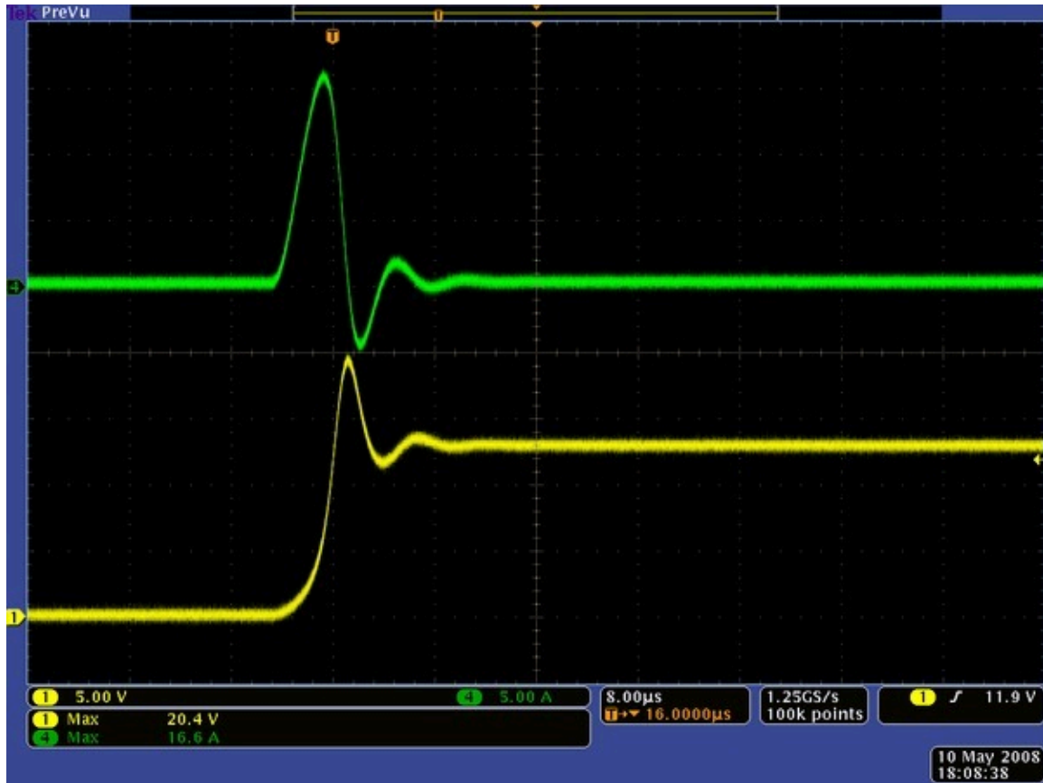
Oscilloscope capture of voltage (yellow) and current (green) when “double-clicking” a Pololu pushbutton power switch connected to a battery.
